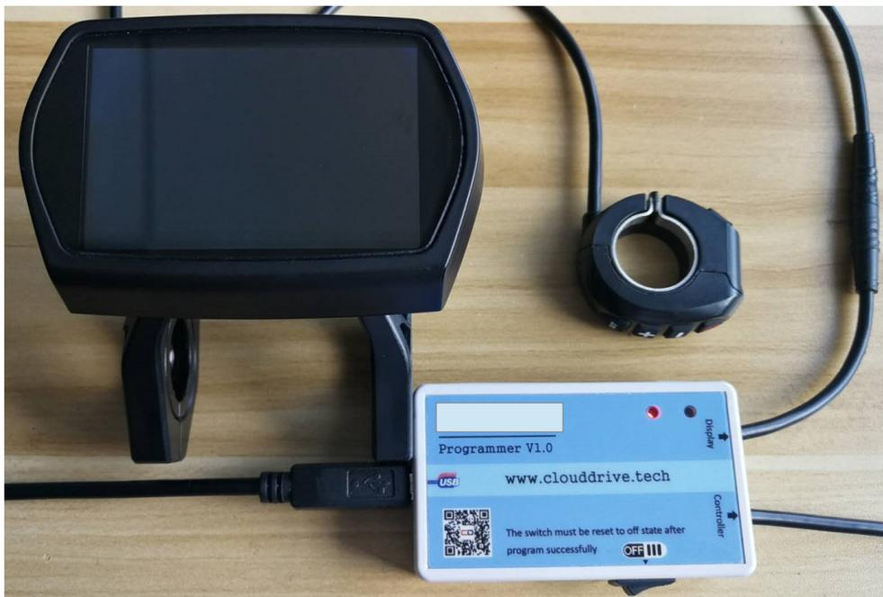
9. Wait for the next progress bar to complete, and the green OK will be displayed, indicating that the instrument's program update is complete. Every time the program is written successfully, the switch of the programmer needs
